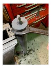
Use a Spanner Wrench to unthread the Glan Nut
