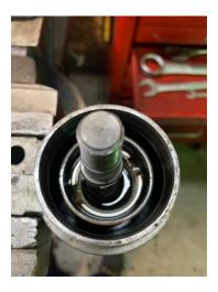
Make sure there is Hydraulic Oil visible to the top of the inner and outer Barrels to ensure that there is enough oil to fully extend the Ram with no air pockets.
