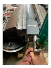
The Final Step to insuring there is no air in the system is to set the Cylinder in a horizontal position and crack the fill cap to release any air then tighten. Once this is complete install the Cylinder onto the Wheel Dolly then test by fully extending then retracting the Ram.
