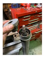
Once the Glan Nut is removed you will see inside the Cylinder Barrel and will find that there is a second Barrel installed inside and the main Piston Cylinder as well.
