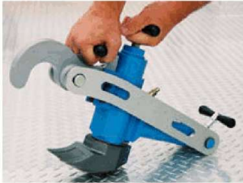
Bead breaker with pin in highest position.
