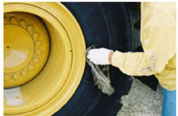
Lubricate with rubber lubricant.
